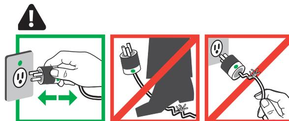
**DANGER!** Electrical cables can be hazardous. Misuse can result in fire or death by electrical shock.
