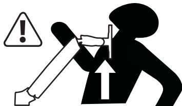
**[EN]** WARNING! Stored Energy Hazard: The arm mechanism is under tension and will move up rapidly, on its own, as soon as attached equipment is removed. For this reason, DO NOT remove equipment unless the arm has been moved to the highest position! Failure to follow this instruction may result in serious personal injury and/or equipment damage!
