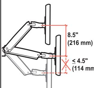
**EN** \* The lower most range of motion for vertical lift is decreased up to 4.5" (114 mm) when arm is adjusted to hold over 20lbs (9 kgs).
