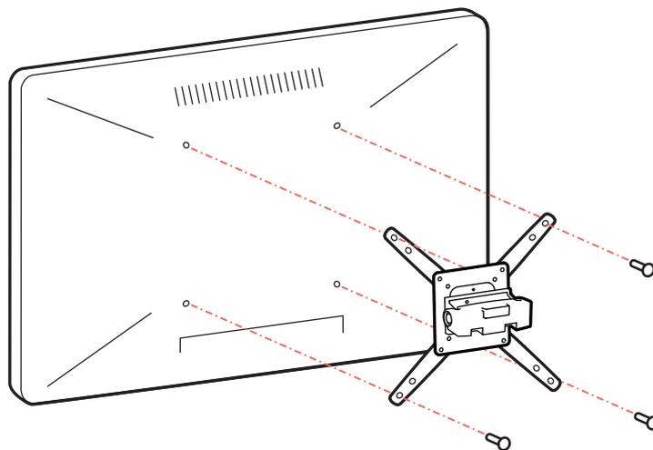
NOTE: To reduce M8 holes for use with M5 screws, or if you have a model with Samsung holder rings, follow the M8M5 KIT instructions on the next page.
