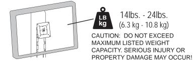
Total weight of monitors when mounted needs to be 14 lbs - 24 lbs (6.2 kg - 10.8 kg)
